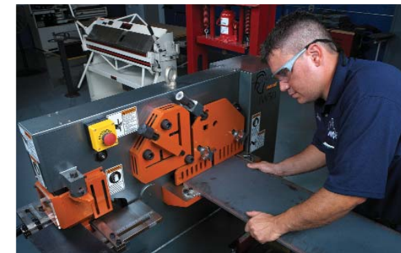
Frank Viscaino on the Hydraulic Ironworker shearing stainless steel. Box and Pan Brake shown in background.
