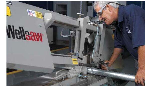
Frank Viscaino, Sr. cutting Schedule 40 solid bar stock for a shaft on the Variable Speed Wellsaw.
